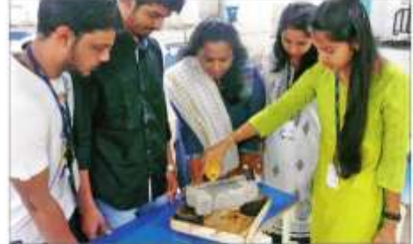
Team of engineering students show new type of mix called pervious concrete that can reduce flooding
