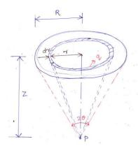
Let q' per unit area = intensity of toad of R be the radius of loaded area
