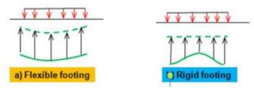
When the footing is flexible, it deforms into the shape of a bowel, with the maximum deflection at the centre. The contact pressure distribution is uniform If the footing is rigid, the settlement is uniform. The contact pressure distribution is minimum at the centre and the maximum at the edges(infinite theoretically). The stresses at the edges in real soil cannot be infinite as theoretically determined for an elastic mass.
