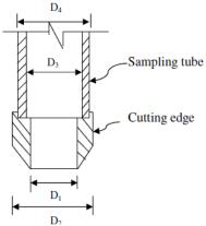
Area ratio  $A_r = \frac{Max. Cross\ sectional\ area\ of\ the\ cutting\ edge}{Area\ of\ the\ soil\ sample}$
