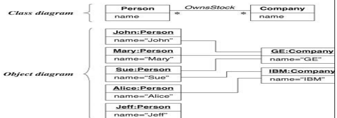
Figure 3.7 Many-to-many association. An association describes a set of potential links in the same way that a class describes a set of potential objects.
