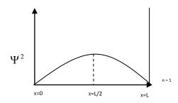
It is seen from the graph that probability density is maximum at the centre for the particle in the first state.
