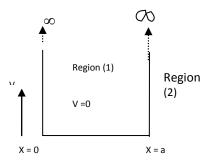
Applying, Schrodingers equation for region (1) as particle is supposed to be present in region (1)
