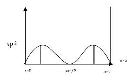
It is seen from the graph that probability density is maximum at x = L / 4 and x = 3L/4 for the particle in the second state.
