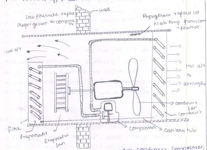
It mainly consists of our evaporator, conduser, compressor, two forms one each for the evaporator 4 conduser units wasually driven by the single motor, capillary, etc.
