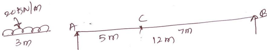
(i) For max -ve S.F load position is as shown below
