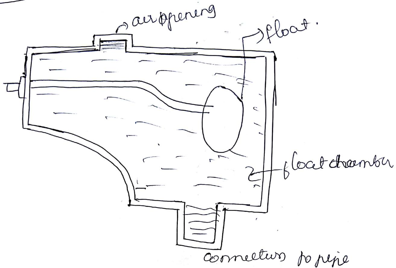
→ In long pipe line, air accumulates at high point of the line which interferes with streamlined flow of water, at such points air valves are provided which remove the accumulated air automatically. This valve has one or two hollow balls inside the float chamber. There are air opening at the top & valves are connected to the main. float chamber normally remains full of water after which the chamber again fill up with water & takes the float up which closes the air opening.
