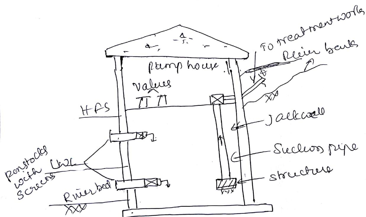
In river intakes water is drawn from upstream side give comparatively better quality of water. They are located sufficiently inside the river so that required demand of water is met in all seasons. It is circular masonry tower of 4 to 7 m in dia. constructed along the bank of river.
