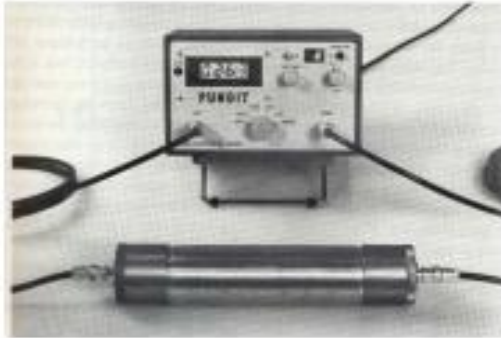
PUNDIT Equipment with flat transducers popularly used for UPV test
