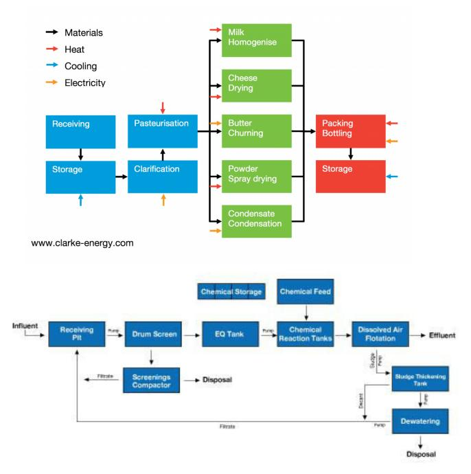
**Dairy Industry Wastewater Treatment**. Producing **milk**, butter, cheese, or yoghurt, using pasteurization or homogenization produces **wastewater** with high levels of BOD and COD loads and must be reduced before being discharged to municipal **treatment** facilities.
