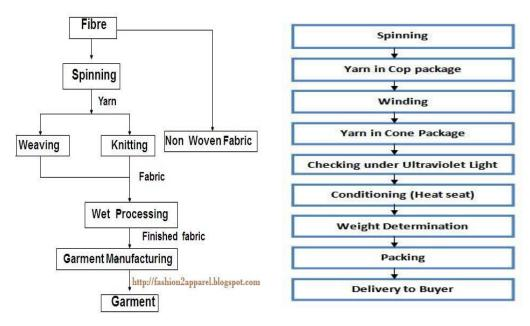
From Raw **Cotton** to **Cotton** Fabrics. The fabric usually used in the clothes we wear is produced through two **processes**: the "**spinning process**," where raw **cotton** is turned into thread, and the "**weaving process**," where the thread is woven into fabric. Here we will explain each **process** in detail using some illustrations.
