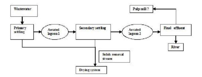
**Paper and Pulp** Manufacture **Wastewater Treatment**- The **paper industry** uses very high volumes of process water for **pulp** preparation and bleaching among other processes. These systems when engineered correctly can dramatically reduce the water usage of a plant through reuse of treated water.
