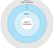
In this OS is divided into number of layers, where one layer is built on the top of another layer. The bottom layer is hardware and higher layer is the user interface.
