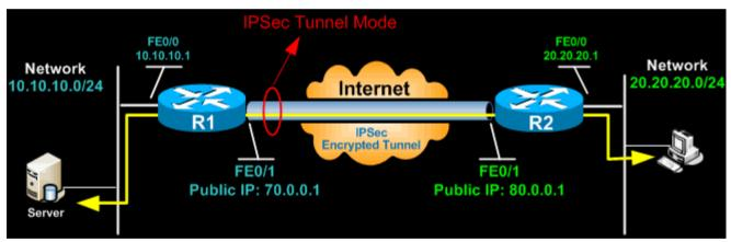
Another example of tunnel mode is an IPSec tunnel between a Cisco VPN Client and an IPSec Gateway (e.g ASA5510 or PIX Firewall). The client connects to the IPSec Gateway. Traffic from the client is encrypted, encapsulated inside a new IP packet and sent to the other end. Once decrypted by the firewall appliance, the client's original IP packet is sent to the local network.
