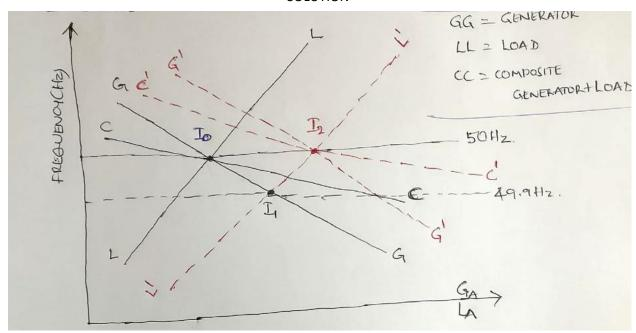
\*. Now the generation characteristic and the load characteristic can be added algebraically to obtain the combined area characteristic to shown by curve CC.
