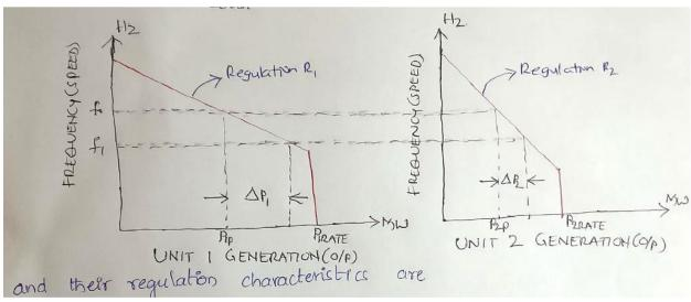
$$R_1 = \frac{\Delta f(p.u.)}{\Delta P_1(p.u.)} = \frac{\Delta f/50}{\Delta P_1/P_1 rate} \quad p.u. \quad D.$$
