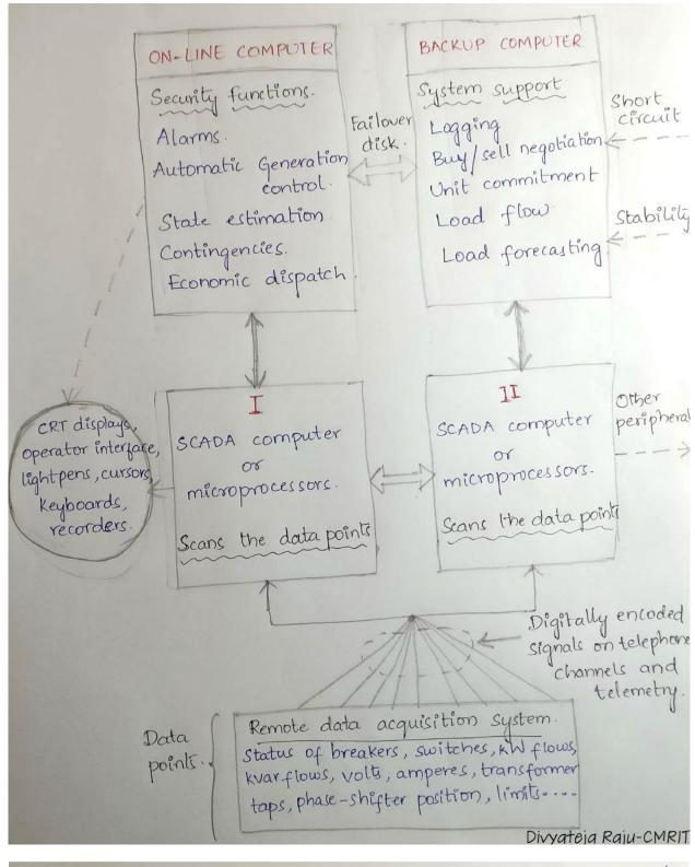
\*. The digital computers are usually employed in fixed cycles. With priority interrupts the computer periodically performs a list of operations.
