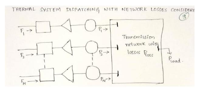
N thermal units serving load through transmission network. \*\*Figure shows all thermal power generation system connected to an equivivalent load bus through a transmission network. \*\* The economic dispatching problem associated with this particular configuration is more complicated than without transmission losses.
