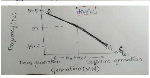
\* The shaft speed and consequently the electrical line frequently changes with load reflected onto the prime mover.
