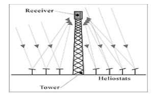
A power tower has a field of large mirrors that follow the sun's path across the sky. The mirrors concentrate sunlight onto a receiver on top of a high tower. A computer keeps the mirrors aligned so the reflected rays of the sun are always aimed at the receiver, where temperatures well *above 1000°C* can be reached. High-pressure steam is generated to produce electricity.
