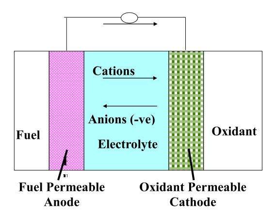
The fuel cell transform hydrogen and oxygen into electric power, emitting water as their only waste product. Every fuel cell also has an electrolyte, which carries electrically charged particles from one electrode to the other, and a catalyst, which speeds the reactions at the electrodes. A single fuel cell generates a tiny amount of direct current (DC) electricity. A converter is used to
