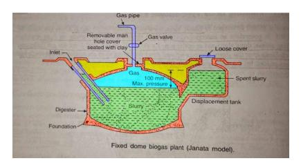
Fixed Dome Type Biogas Plant - Janata Model
