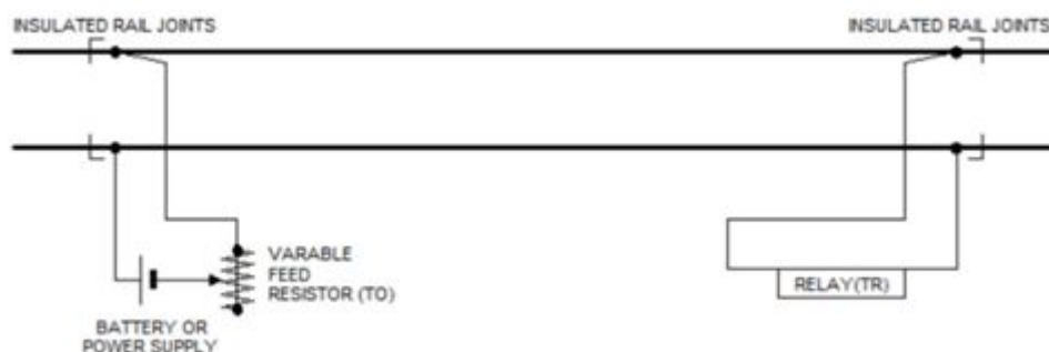
Figure 3.3: Track Circuit mechanism
