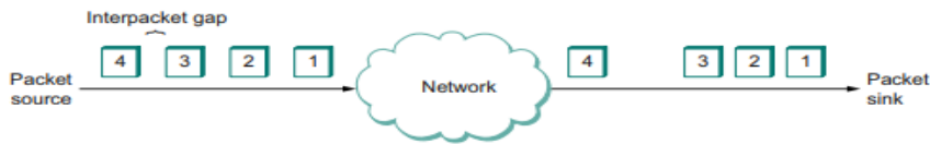
■ FIGURE 1.20 Network-induced jitter.
