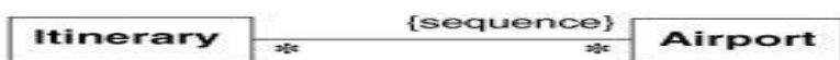
Figure 3.16 An example of a sequence. An itinerary may visit multiple airports, so you should use {sequence} and not {ordered}. Object-Oriented Modeling and Design with UML , Second Edition by Michael Blaha and James Rumbaugh. ISBN 0-13-1-015920-4. © 2005 Pearson Education, Inc., Upper Saddle River, NJ. All rights reserved.
