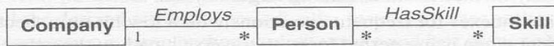
Figure 15.5 Analysis model for person skills. Derived data is undesirable during analysis because it does not add information.
