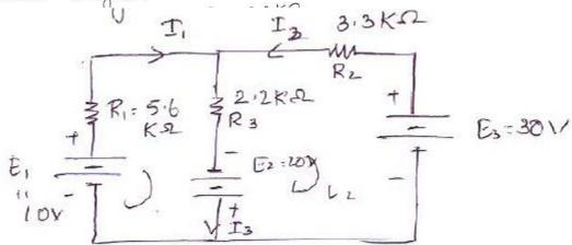
Applying K.CL at node A I, + I2 = I3 Applying K.V.L to loop L1. (5600) I, +(2200) I<sub>3</sub> = 30 \$(5600) I, + (2200) (I,+I2) = 30  $7800I_1 + 2200I_2 = 30 \longrightarrow (1)$ Applying K.V.L to Loop Lz (-3300)  $I_2 + (-2200)(I_3) = -30-20$  $(-3300)_{12} + (-2200)_{1} + (1) = -50$ -2200 I, -5500 I2 =-50 -> (2) Solving (1) & (2) We get It = 1.4 MA I2 = 8:51 MA I3 = I2-I1 = 7 . 11 MA
