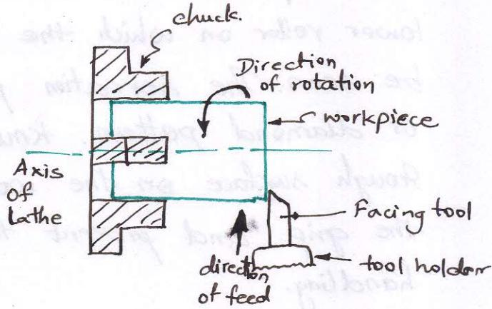
In facing operation, the direction of feed given is perpendicular to the axis of the lathe. The workpiece is held in the chuck and the facing tool is fed either from outer edge of the workpiece progressing towards the center or vice-versa. The cutting tool is held by a tool holder in a tool post. Axial movement of the
