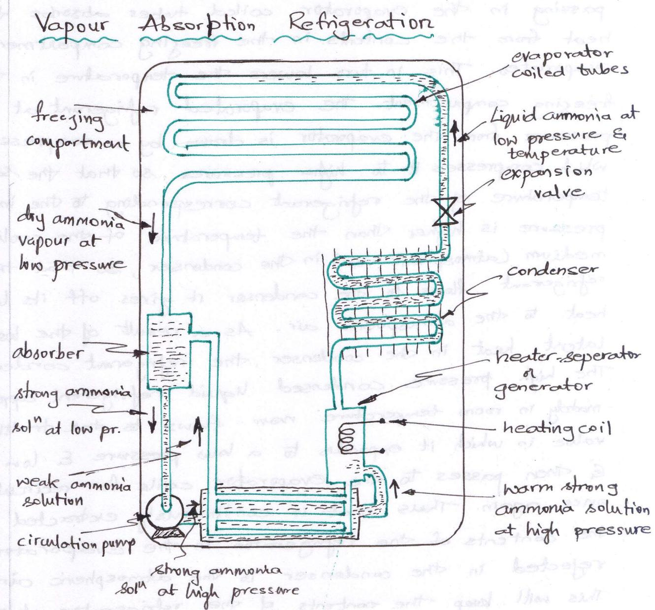
A vapour absorption system makes use of the ability of a substance, called absorbent to absorb large volumes of the vapour of a refrigerant even when cold, and reduce it to a liquid, and subsequently give off its vapours when heated.
