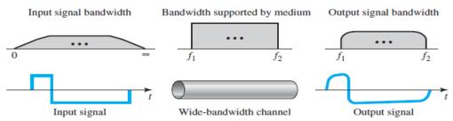
An example of a dedicated channel where the entire bandwidth of the medium is used as one single channel is a LAN.
