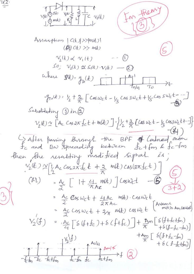
SSB-SC Filtering method る。 Ds B 1/2 Squ(I+fc) - 1/2 sgn(f-fc) Helt) / 1 Sqn (f-fc)] YDSB(f), I [AcM (ftfc)+Mlf-fc)] XSSB(f) = 1 Ac [M(J+fc) Sqn(J+fc) +M(f-fc) Sgn(I+fc) - 4 Ac [M(f+fc) sqn(f-fc) +M(f-fc) sqn(f-fc)]3 = 1 Ac [M(f+fc)x=sgn(f-fc)] + LAC [M(J-fc) \* Sgn(ftfc)]
