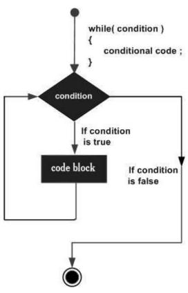
Here, key point of the *while* loop is that the loop might not ever run. When the condition is tested and the result is false, the loop body will be skipped and the first statement after the while loop will be executed.
