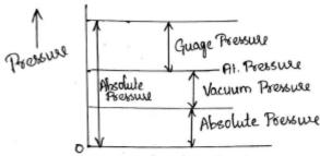
Guage Pressure is measured above the atmospheric pressure.
