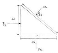
Consider a Widge Hawld Element of dimension de, dy and 2 let, Pro ty and P2 be the Pressure applied in x-3 y and in Inclined 2 direction.
