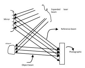
The given object, mirror and photographic plates are arranged as shown in the figure .An expanded laser beam is directed on this arrangement in which a part of the beam is incident on the mirror and the rest falls on the object.
