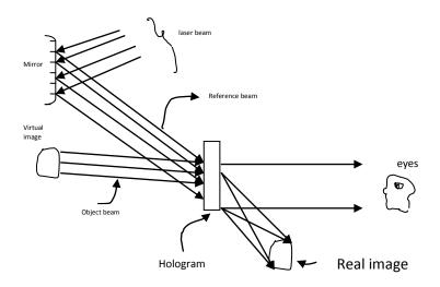
The image of the object is reconstructed by passing the reference beam from the same laser through the hologram ,which is oriented with respect to the reference beam .The reference beam is diffracted and two images of the object , real image and virtual image are seen. [2]
