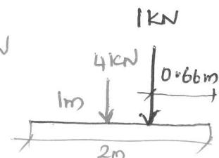
5(b) Determine the support reactions for the beam shown in fig 5(b).
