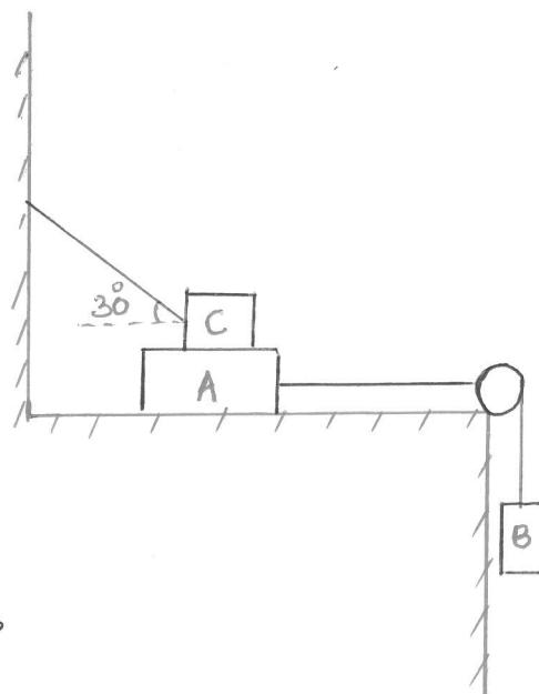
As block A moves towards right, frictional forces act on it towards left on both of its faces. Hence the frictional force acting on the block C must be in opposite direction ie towards the right.
