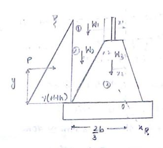
Base width 'b' of the weis is fixed by stability against overlanding. For stability succeltant should lie within the middle third of the base. At central cond resultant should pass through o' at ab from us edge (fig).
