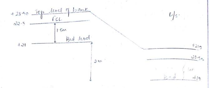
a) Design of trapezoldal notch: Let us assume two notches are provided, to pass the discharge from cys to d's Section.
