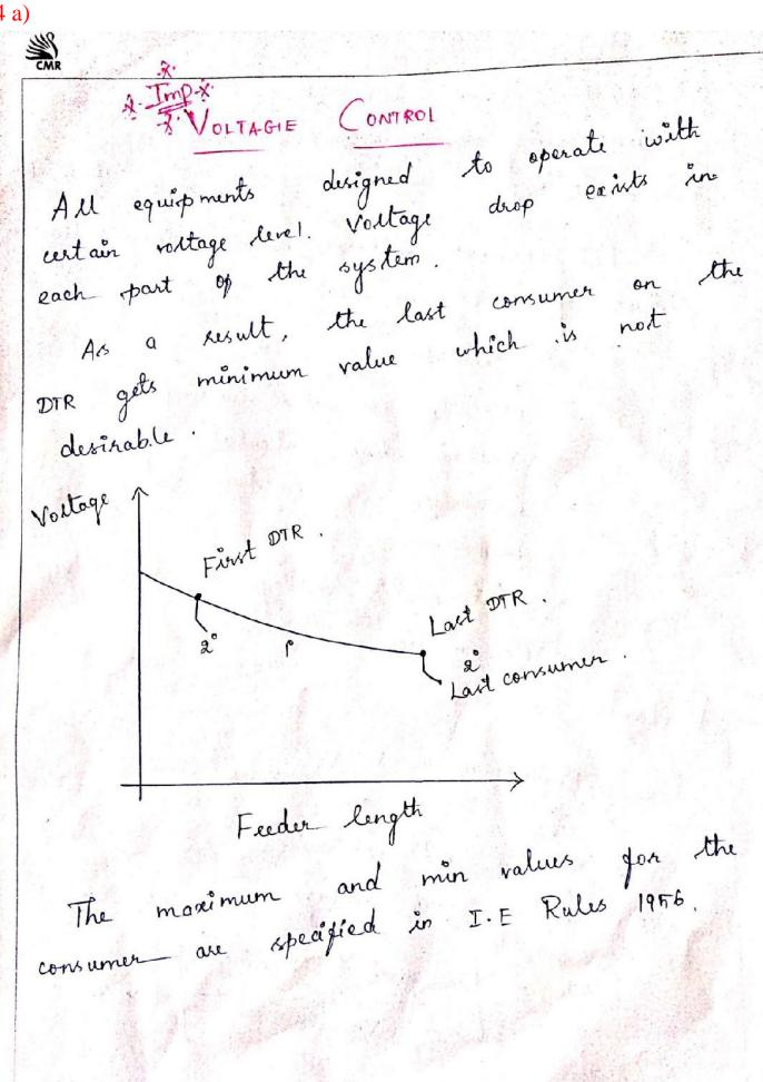
→ Voltage drop and loss depend upon line impedance as well as loading.
