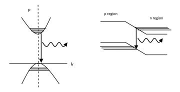
The first laser action was observed in a GaAs junction(8400Å) which is a direct gap semiconductor.
