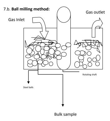
Principle: Small hard balls are allowed to rotate inside a container. The bulk sample is sprinkled. The steel balls crush the solid into nano crystal.
