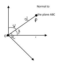
Let ABC be one of the parallel planes represented by the Miller indices [h,k,l]. Let its intercepts be x,y,z. Imagine another plane passing through the origin O .OD is the perpendicular from O to the plane ABC and OP is the interplanar distance. Let the angle made by OP with X,Y and Z axis be  $\alpha$ ,  $\beta$  and  $\gamma$  respectively.
