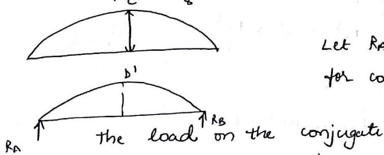
$$\begin{aligned} &= \text{Area of the load diagram} \\ &= \frac{2}{3} \times (A'B') \times (C'D') \\ &= \frac{L}{3} \times L \times \frac{wL^2}{8EI} \\ &= \frac{WL^3}{12EI} \end{aligned}$$
