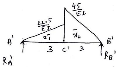
$$\begin{aligned} * \text{ Load b/w } A' \text{ & } C' &= \text{Area of the load dia} \\ &= \frac{1}{2} \times A_{C'} \times C_{D'} \\ &= \frac{1}{2} \times 3 \times \frac{22.5}{EI} \end{aligned}$$
