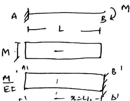
i. Slope @ B  $\theta_B = \text{load } A'B'C'D'$
