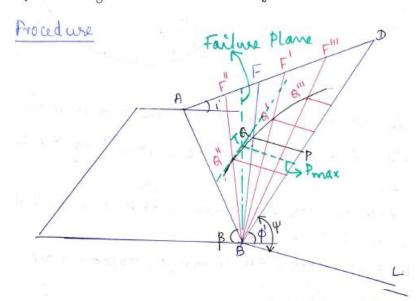
From B, a line BD is drawn at an angle  $\phi'$  to the base thre weight of the wedge is flotted along line is also known as the weight line.
