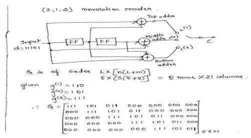
6 Consider a (3,1,2) convolution code with  $g^{(1)}=(110), g^{(2)}=(101)$  and  $g^{(3)}=(111)$ . Find the code-word corresponding to the information sequence (11101) in *Time Domain* approach and *Transform Domain* approach
