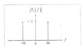
b Determine and sketch the spectrum of the resulting DSB-SC AM signal, identify the upper and lower sidebands in the spectrum.
