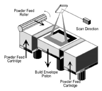
The SLS process is based on the following two principles:
