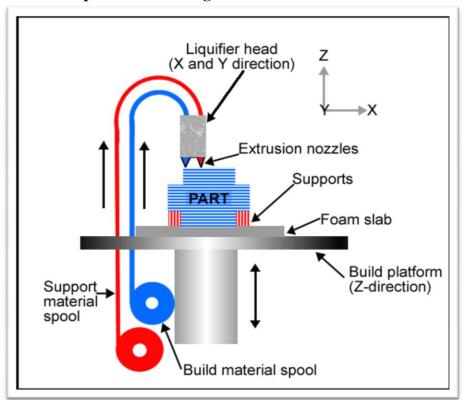
In this patented process [12], a geometric model of a conceptual design is created on a CAD software which uses IGES or STL formatted files. It can then imported into the workstation where it is processed through the QuickSlice® and SupportWork $_{\text{TM}}$  propriety software before loading to FDM.
