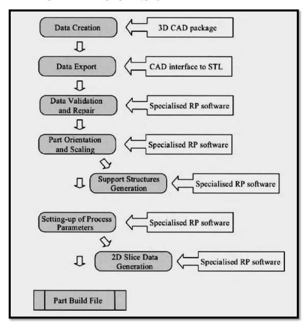
(1) A model or component is modeled on a Computer-Aided Design/ Computer-Aided Manufacturing (CAD/CAM) system. The model which represents the physical part to be built must be represented
