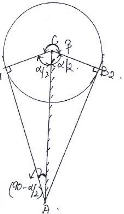
$$\text{Time Ratio (TR)} = \frac{\text{Time of cutting stroke}}{\text{Time of return stroke}} = \frac{360^\circ - \alpha}{\alpha} = \frac{360^\circ - 132.8^\circ}{132.8^\circ}$$
