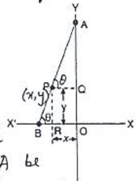
(b). Let us take OX and OY as horizontal and vertical axes and let the link BA be inclined at an angle  $\theta$  with the horizontal. P has the co-ordinates as  $(x, y)$ .
