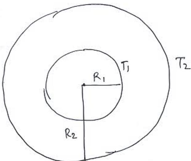
Assuming that only radial heat conduction takes place at steady state and there is no heat generation.
