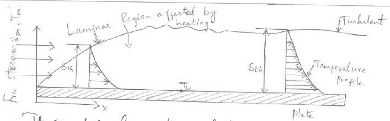
It is defined as the distance from the boundary in which the temperature difference reaches 99% of the initial temperature.
