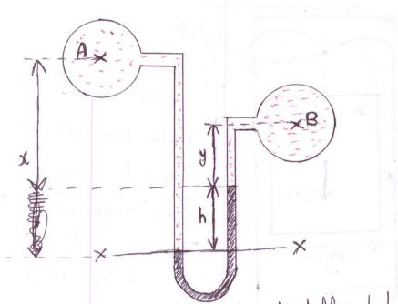
Let two pipes A and B be at different levels and contain different fluids.
