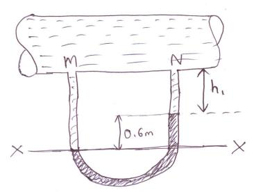
$P_{X-X}(left) = P_{X-X}(right)$   $P_{m} + S_{wg}(h_{1} + 0.6) = P_{N} + S_{wg}(h_{1}) + S_{Hy}g(0.6).$   $P_{m} - P_{N} = S_{wg}h_{1} + S_{Hy}g(0.6) - S_{wg}h_{1} - S_{wg}0.6$   $P_{m} - P_{N} = 13600 \times 9.81 \times 0.6 - 1000 \times 9.81 \times 0.6$   $P_{m} - P_{N} = 74.16 \times N/m^{2} = 74163.6 \times N/m^{2}$
