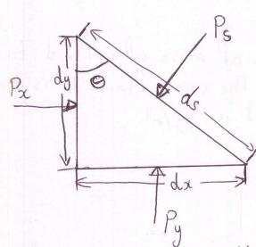
Consider an arbitary Pluid element of wedge shape in a fluid mass at rest. Let the width of the element L'ar to paper be unity.
