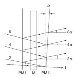
Partial mirror can be used to multiply the number of Isochromatics fringes if one partial mirror is placed parallel to the photo elastic model and the other partial mirror is placed slightly inclined
