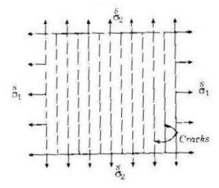
In this case, only one set of cracks forms, and they are perpendicular to  $\sigma_1$ . These cracks indicate the principal stress direction of  $\sigma_2$ , and, as a consequence, the cracks represent stress trajectories, or isostatics.
