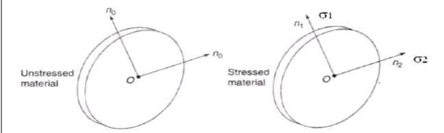
fig 1 shows a unstressed thin disc of a photo-elastic model. The refractive index of this material in any direction is  $n_0$ . This thin disc is subjected to loads such that the principal stresses developed at a point o are  $\sigma_1$  and  $\sigma_2$  as shown in fig 2. The refractive index of material changes in the direction of  $\sigma_1$  to the value  $n_1$  and  $n_2$  in the direction  $\sigma_2$ . These changes in refractive idiocies are linearly proportional to the stresses.
