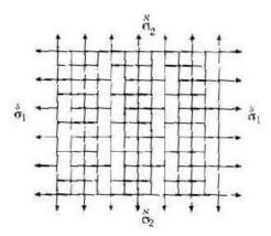
For this two families of cracks can form. The first set of cracks due to  $\sigma_1$  forms perpendicular to  $\sigma_1$  and parallel to  $\sigma_2$ . When the stress level of  $\sigma_2$  becomes sufficiently high, a second family of crack will form perpendicular to  $\sigma_2$  and parallel to  $\sigma_1$ .
