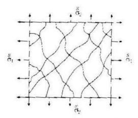
When  $\sigma_1 = \sigma_2$  at any point on the body, the stress system is said to be isotropic and every direction is a principal direction. If the values of  $\sigma_1$  and  $\sigma_2$  are sufficiently high, the coating will fail; however, the crack pattern produced will be random in character. Crack pattern of this form are often referred to as craze patterns since the crack have no preferential direction.
