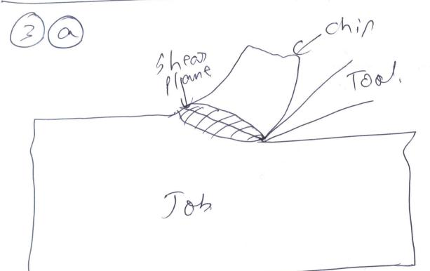
The hool is forced to move against the figh during cutting, during this the tool compresses that job directly infoont of the cutting edge. Because of this for stress exerted on the job, the job is going to slip along the slip
