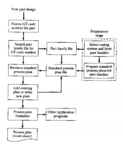
A retrieval CAPP system, also called a variant CAPP system, is based on the principles of group technology (GT) and parts classification and coding. In this type of CAPP, a standard process plan (route sheet) is stored in computer files for each part code number. Before the system can be used for process planning, a significant amount of information must be compiled and entered into the CAPP data files. This is the "preparatory phase:' It consists of the following steps:
