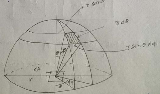
cousider radiation emitted from an elemental black surface from area dA & temp Ti Energy will emitted in all the directions on the entire hemisphen.
