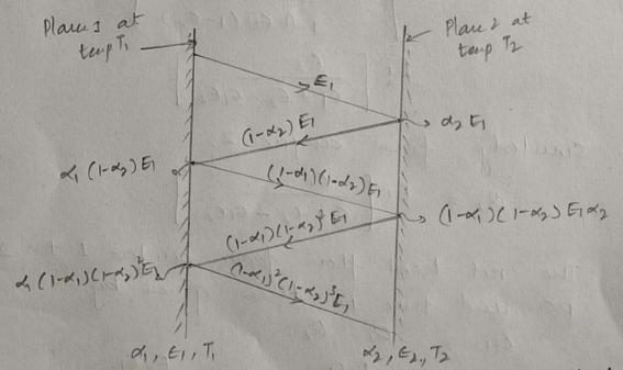
The serface I emits radiant energy Es which stocker the surface 2 and the semainder (1-x2) E is replected back to surface I. on reaching surface 1, a part x1 (1-x2) E1 1's absorbed and remainder
