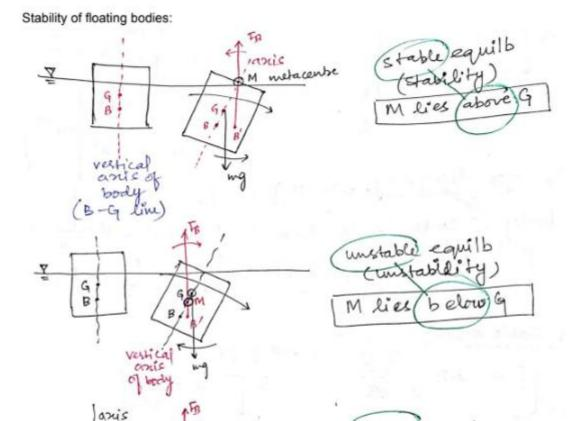
Metacentric height is significant in deciding dimensions of a prototype so that it can be made stable while floating in water. We have to ensure that GM > 0.
