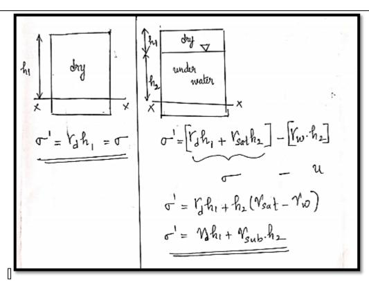
Effective stress is the difference of total stress and fore router pressure. It cannot be measured directly like total stress on fore router fression. It can only be computed from and r.
