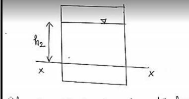
Of the soil is dry fore water frassure = 0 Pore water frassure can be measured by a piezometer
