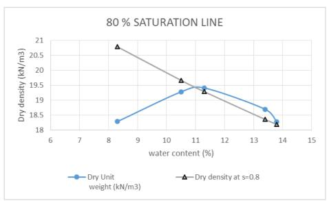
iii. Void ratio and degree of saturation at OMC.
