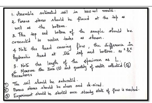
4. Throughout the experiment the grate of inflow of water should be equal to grate of outflow of water in the head difference is always kept constant.
