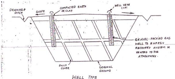
The movement of landfill gases through adjacent soil formations can be controlled by constructing barriers of materials that are more impermeable than the soil. Some of the landfill sealants that are available for this use are Betonites, illites, Kaolinites, sodium carbonate, silicates, pyrophosphate, polymers, rubber latex etc. out of these, the compacted clay is most common.
