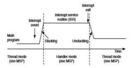
CONTROL[1]=0: Both Thread Level and Handler Use Main Stack.
