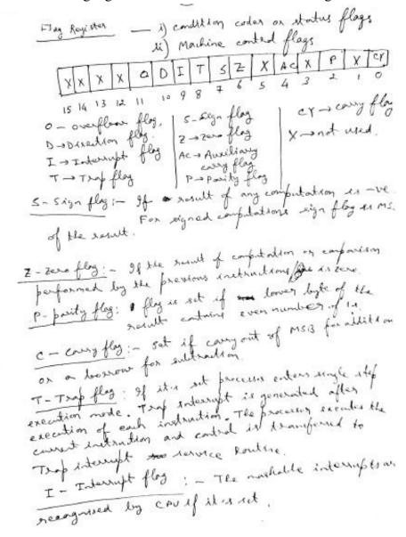
D-Direction flog: If I this lit is 'O' the else, is processed beginning from the lowest address, to the lighest address, i.e. autoincrementating made.
