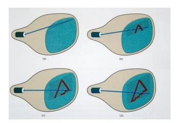
The electron beam is swept across the screen one row at a time from top to bottom.
