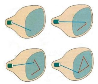
When operated as a random-scan display unit, a CRT has the electron beam directed only to those parts of the screen where a picture is to be displayed.
