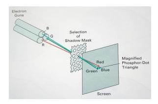
The most predominant type of display has been the Cathode Ray Tube (CRT) Various parts of a CRT:
