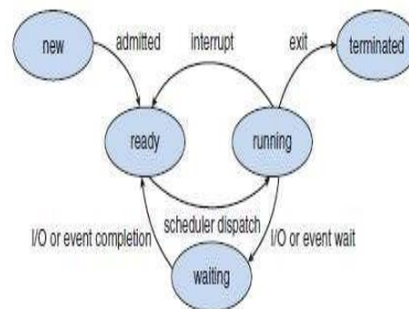
Figure 5 Diagram of process state
