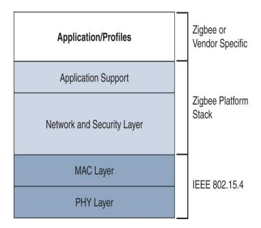
Zigbee is a wireless technology developed as an open global standard to address the unique needs of low-cost, low-power wireless IoT networks The Zigbee standard operates on the IEEE 802 15 4 physical radio specification and operates in unlicensed bands including 2 4 GHz, 900 MHz and 868 MHz
