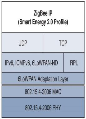
The main functions of the network layer are to enable the correct use of the MAC sublayer and provide a suitable interface for use by the next upper layer, namely the application layer
