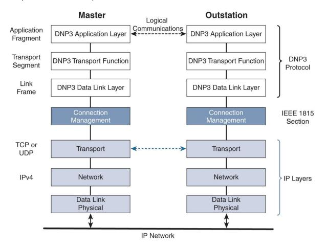
DNP3 is a communications protocol used in SCADA and remote monitoring systems — It is widely used because it is an open protocol, meaning any manufacturer can develop DNP3 equipment that is compatible with other DNP3 equipment
