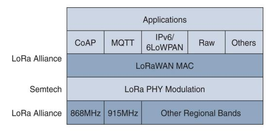
oRa uses license-free sub-gigahertz radio frequency bands like 169 MHz, 433 MHz, 868 MHz (Europe) and 915 MHz (North America) LoRa enables long-range transmissions (more than 10
